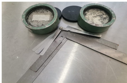
Figure 1. Equipment required for the endorsement of concrete cylinders in accordance with ASTM-C-1231
